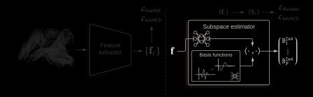
• Subspaces encode change of motion over time  $\Rightarrow$  time-dependent basis
